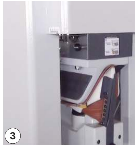
Step 3. Press the START buttons at the same time and release the pedal to complete the procedure. The machine will revert to its initial position after the end of the setting time.
