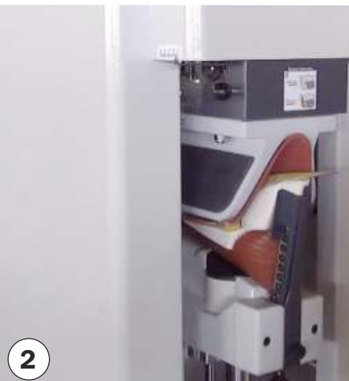
Step 2. Press the pedal to hold the upper (Figure 2). Before continuing the procedure be sure that the upper is in the right crimping position.
