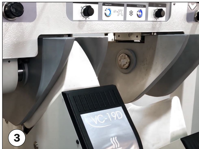
Step 3. Press the START buttons simultaneously and release the pedal to complete the procedure. The machine will revert to its initial position after the end of the setting time.
