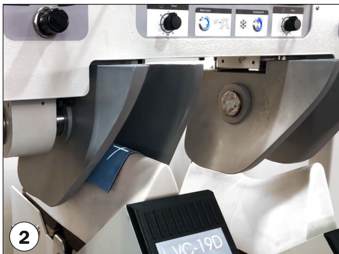
Step 2. Press the pedal to hold the vamp (Figure 2). Before continuing the procedure be sure that the vamp is in the right crimping position.
